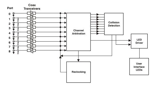
Figure 2-1. DNH-6800 Block Diagram Flow
